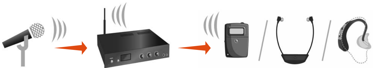
Assistive listening systems includes microphone, transmitter, and receivers
